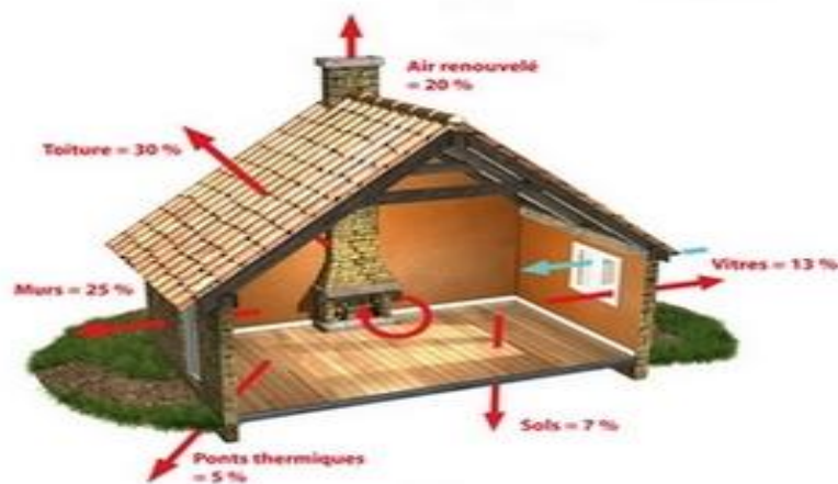
Fig. 4 Proportion of heat loss through different parts of the building fabric (CAPEB, 2009)
